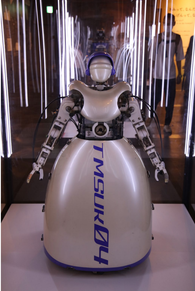
TMSUK04 1999 (TMSUK) Humanoid tele-operated robot which can be controlled remotely via PHS line.
