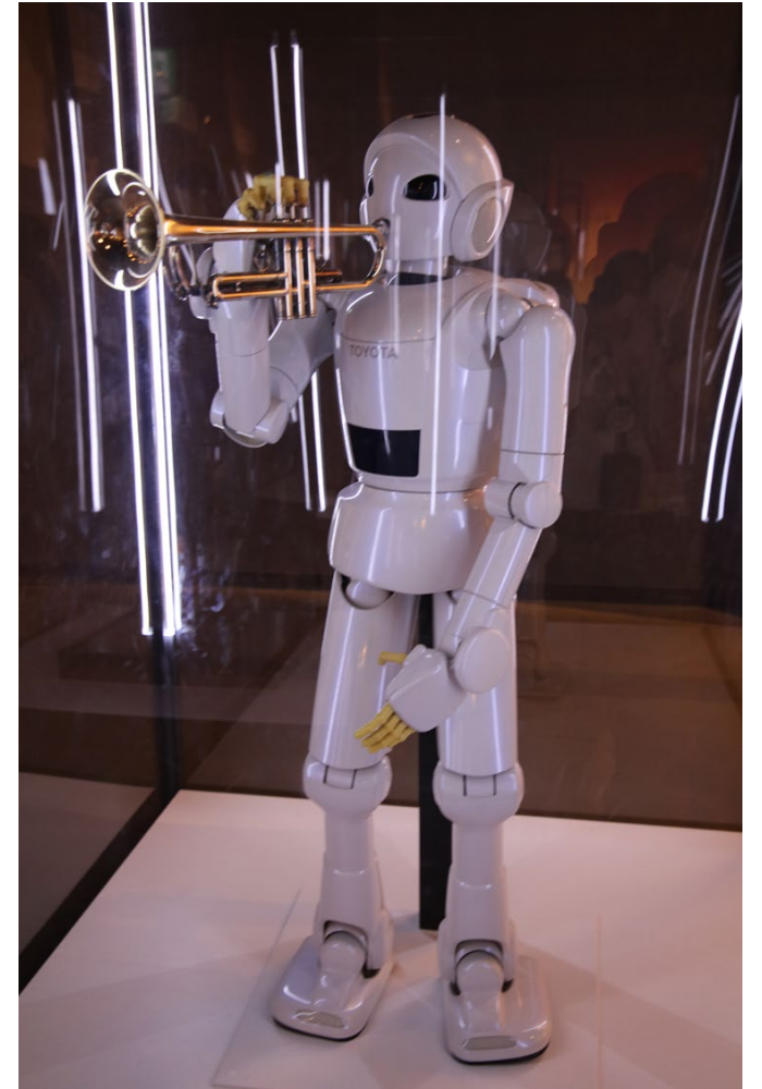
Partner Robot Harry 2004 (TOYOTA) This robot can play the trumpet through delicate mouth, hand, and finger movements.
