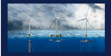
Mooring and cable equipment is a key cost driver within floating wind.
